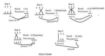
Initially the LSB digits on the both numbers of the line are multiplies and added with the carry from the previous step. This generates one of the bits of the result and carry. This carry is added in the next step and the process goes on likewise. When there are more lines in one step, all the results are added to previous carry.
